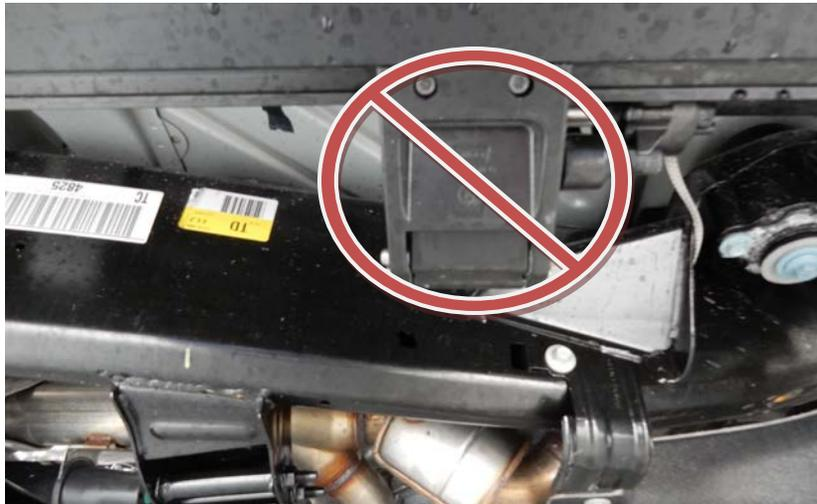
**Caution:** This vehicle is equipped with stow away running boards. Avoid all contact when jacking.
