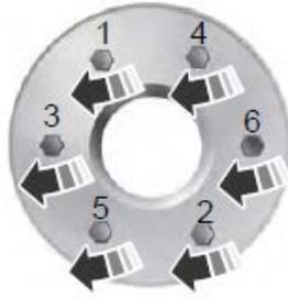
**Tighten lugnuts in the pattern shown above**
