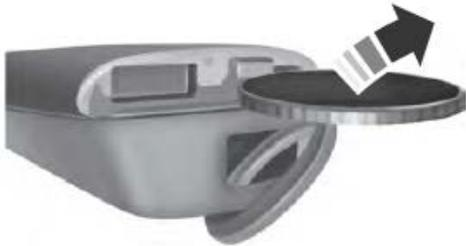
2. Twist a thin coin under the tab hidden behind the key blade head to remove the battery cover. Do not use the key blade to remove the cover or you could damage it.
