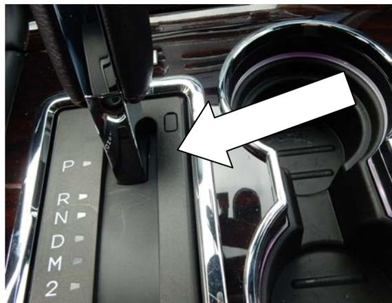
2. Locate the shift interlock access cover on the passenger's side of the shifter.
