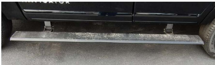
**Running Boards Deployed**
