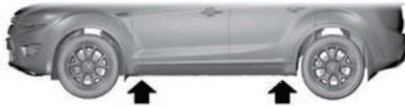
Use the jacking points shown above. Place the jack in its proper location on the frame. Observe all standard jacking precautions and ensure that the vehicle is on firm, level ground and that the wheels are chocked. As the jack comes in contact with the vehicle body, ensure that it is contacting the correct location on the vehicle.
