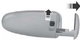
Slide the release on the back of the remote to access the key blade.
