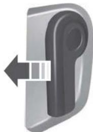
To open the hood: pull the hood release handle located under the left-hand side of the instrument panel and find the secondary release lever, which is located under the front of the hood, near the Lincoln badge.
