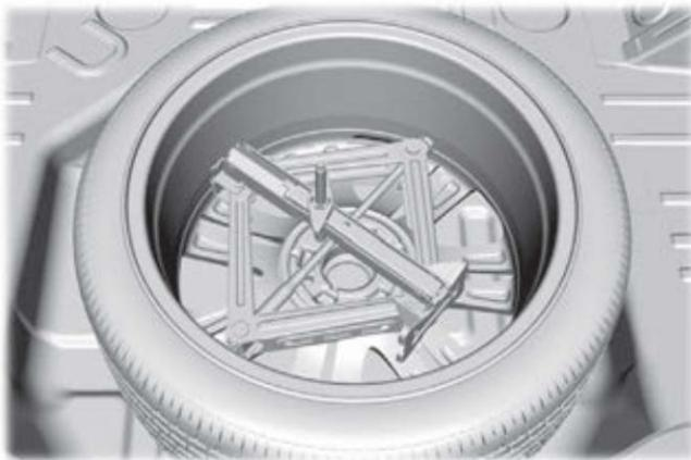
The spare tire and factory tools are located in the trunk, under the package shelf in the wheel well.
