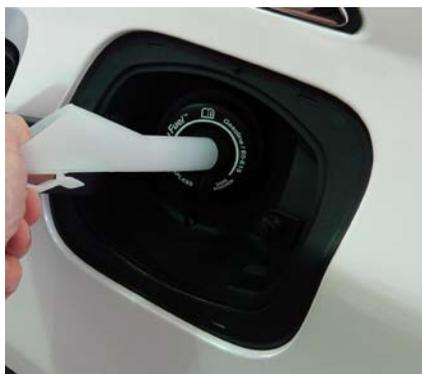
Locate the portable funnel that comes with the vehicle. The fuel filler funnel is located in the spare wheel storage tray. Carefully insert the funnel into the capless fuel system to add fuel.
