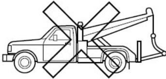
**Ford Motor Company has not approved a slingbelt towing procedure. Vehicle damage may occur if towed incorrectly, or by any other means.**
