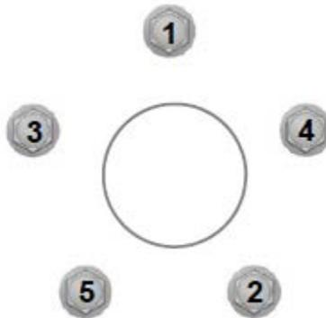
**Tighten lugnuts in the pattern shown above**
