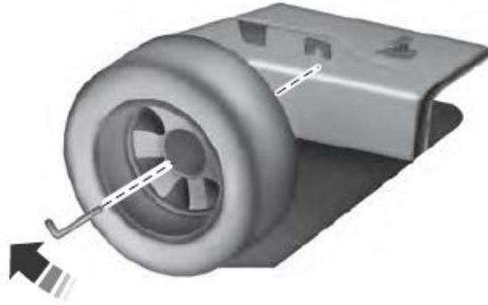
If the road wheel you removed cannot be secured in the wheel well area, remove the L-shaped bolt from the external pocket of the felt bag. With the third row seat in the raised position, stand the flat tire in the rear of the vehicle with the tire's valve stem facing the rear of the vehicle. Fasten the flat tire to the vehicle by inserting the L-shaped bolt through one of the lug bolt holes in the wheel. Turn it clockwise into the threaded hole in the vehicle until the tire is secured.
