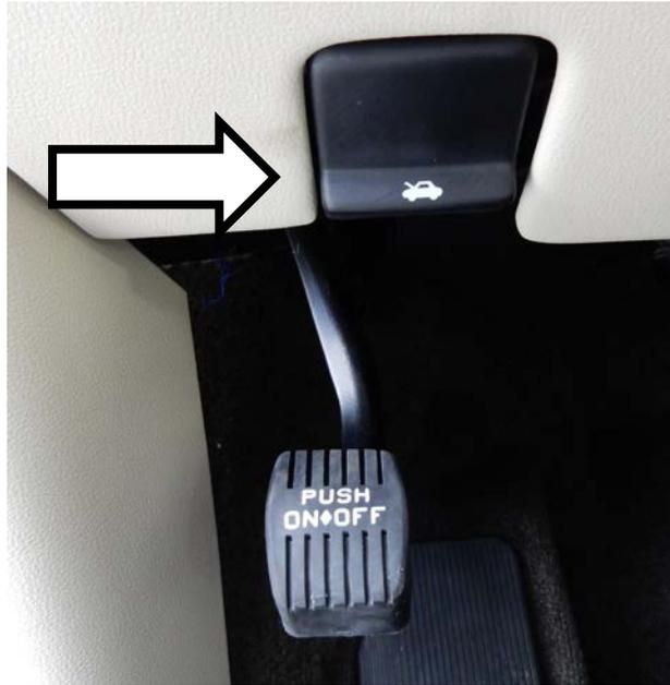
To open the hood: pull the hood release handle located under the far left-hand side of the instrument panel.
