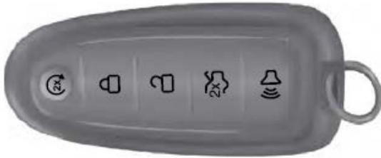
The intelligent access keys operate the power locks and the remote start system. The key must be in the vehicle to activate the push-button start system.
