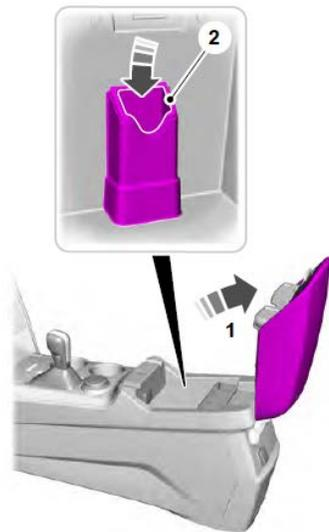
2. Insert the passive key into the backup slot.
