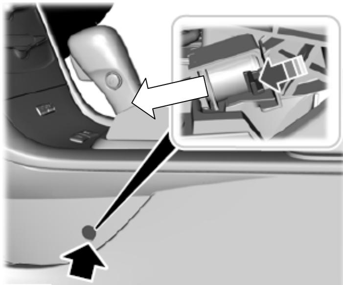
2. Carefully remove the access plug on the side of the center console.
