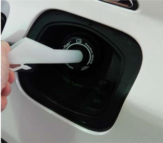
Press the center-rear edge of the fuel filler door and release to open. Locate the portable funnel that comes with the vehicle. The funnel is located in the trunk. Carefully insert the funnel into the capless fuel system to add fuel.
