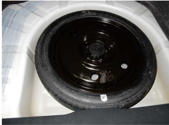
The spare tire and factory tools are located in the trunk, under the package shelf, in the wheel well.
