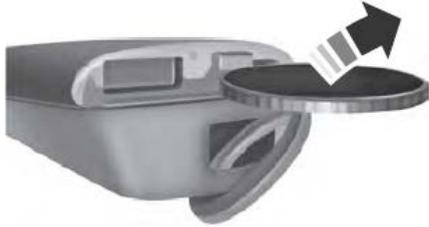
1. Remove the key blade from the transmitter.
