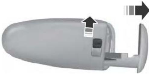
**Removable Key Blade** The intelligent access key also contains a removable mechanical key blade that you can use to lock or unlock the driver door.
