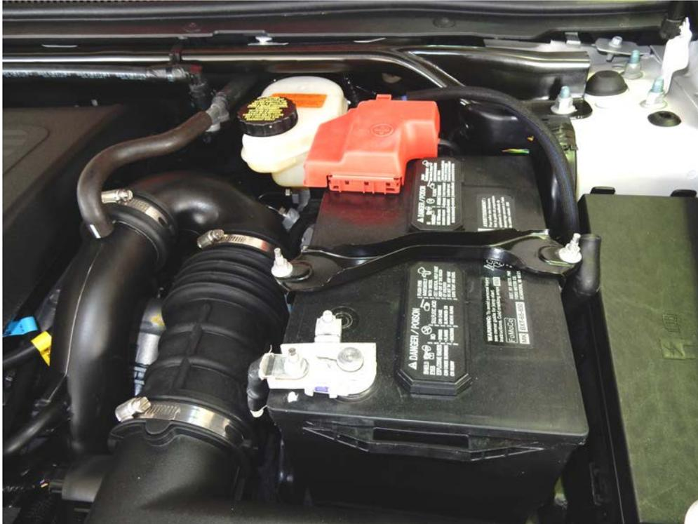
**The battery is located on the driver's side of the engine compartment.**
