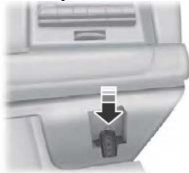
2. With the key in this position, press the brake pedal, then the button to switch the ignition on and start the vehicle.
