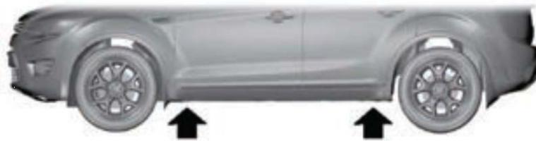
Use the jacking points shown above. Place the jack in its proper location. Observe all standard jacking precautions and ensure that the vehicle is on firm, level ground and that the wheels are chocked. As the jack comes in contact with the vehicle body, ensure that it is contacting the correct location on the vehicle.
