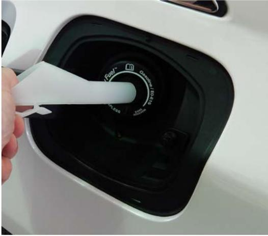
Locate the portable funnel that comes with the vehicle. The fuel filler funnel is located in the spare wheel storage tray. Carefully insert the funnel into the capless fuel system to add fuel.
