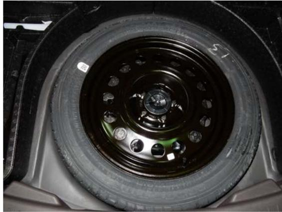
The spare tire and factory tools are located in the rear cargo area under the package shelf, in the wheel well.
