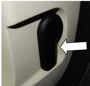
To open the hood: pull the hood release handle located under the left-hand side of the instrument panel and find the secondary release lever, which is located under the front of the hood, near the Lincoln badge.
