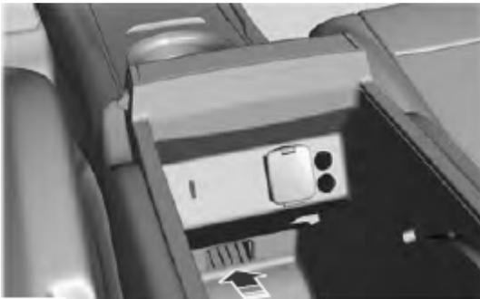
2. Slide the remote into the back-up slot.
