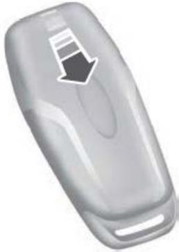
1. Slide the release on the back of the remote control and pivot the cover off.
