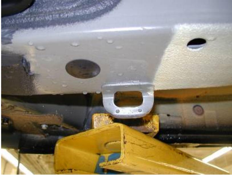
*Figure 3 (front tie down slot)*
