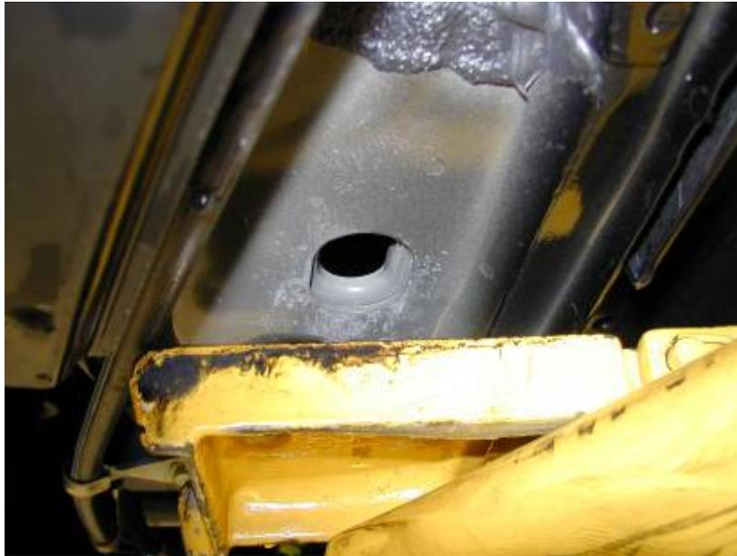
*Figure 4 (rear tie down slot)*
