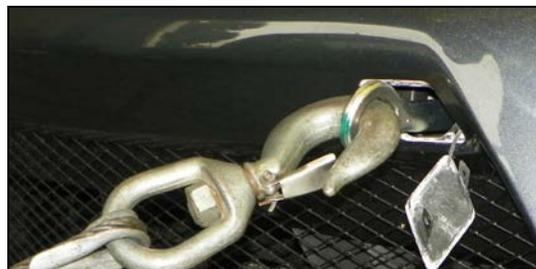
Before loading, ensure that the transmission is in “Neutral” and the ignition switch is in position to unlock the steering. When loading, remember that the eye bolts are designed for a straight ahead pull within a 20 degree window, so stop the vehicle as the winch wire rope begins to pull downward. To prevent too much downward pull you will need to keep the leading edge of the vehicle about 2 feet from the winch drum.
