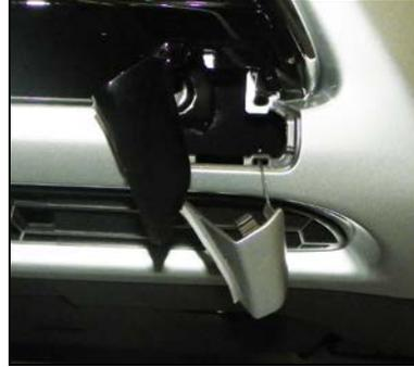
To install the eye bolt correctly on this vehicle, start by carefully removing top half of the two piece eyelet receiver cover from the bumper. The cover is easily damaged. Work carefully. If a sharp, metal object like a screwdriver is used as shown above, use a cloth or piece of paper to protect the painted surfaces from scratches.
