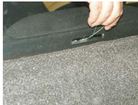
Pulling on the cable unlatches the rear cargo area cover.
