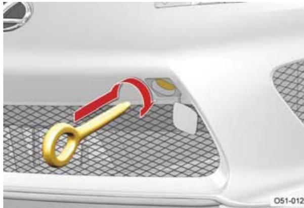
Attach your winch line hook to the eyelet ensuring there is no contact between the hook and the painted surface. Leave the winch line attached to the installed towing eyelet throughout the loading, transporting and unloading processes.
