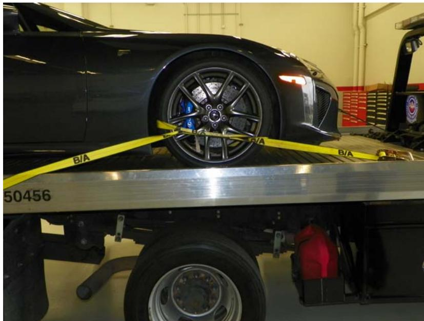
Due to the inset of the wheels and the width of the body, careful routing of the straps is important to avoid contact with the painted surface. You will notice in the two pictures above, the strap end that is traveling toward the middle of the car is routed on the outside of the bedrail. This was done to prohibit strap contact with the body of the vehicle. The end of the strap is secured into the bed tie-down slot from the underside.
