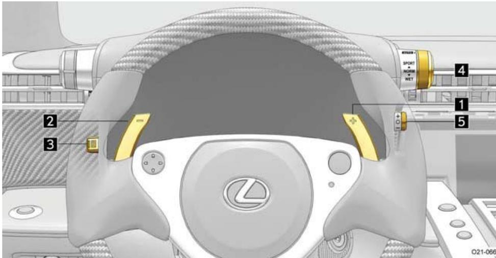
To shift the transmission into Neutral (“N”), turn the ignition to the ON position and pull both shift paddles toward you.
