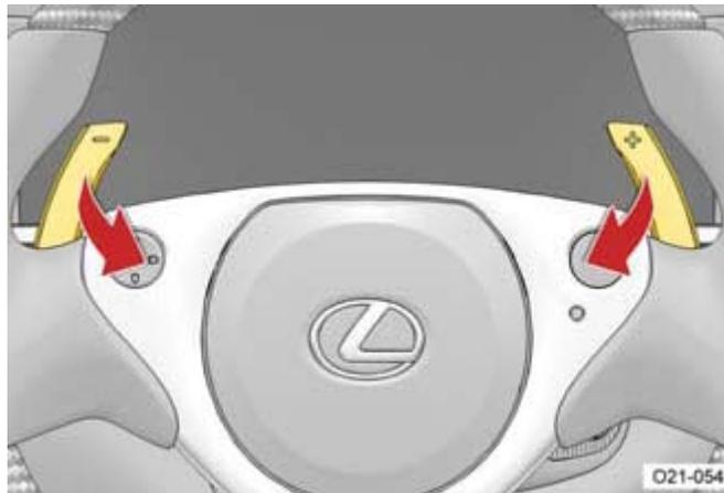
To shift the transmission into Drive (D1 or 1<sup>st</sup> gear) pull the Upshift paddle toward you.
