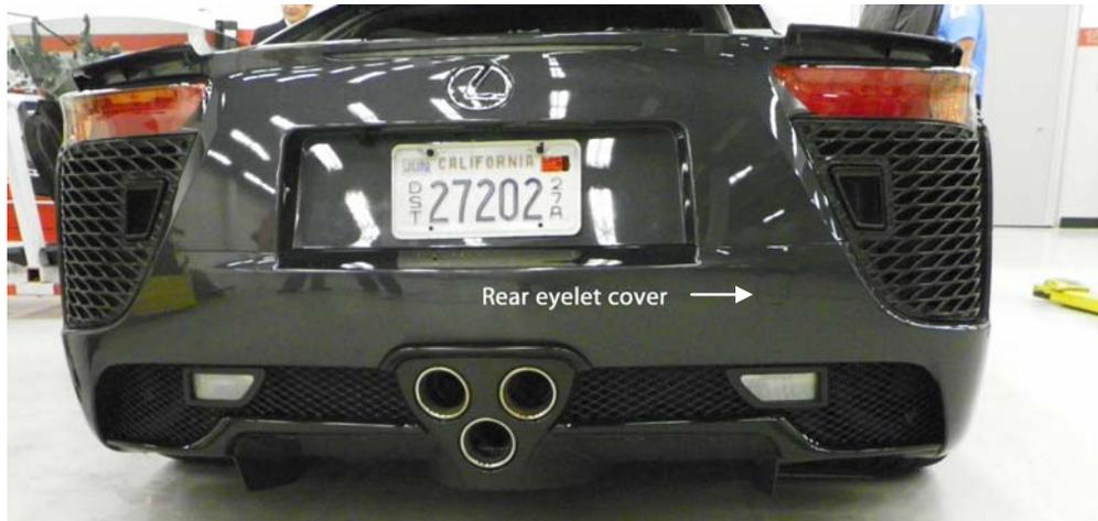
Although the receiver cap cover has a string-type piece that holds it to the vehicle when it is removed, it is always a good idea to remove the assembly completely from the bumper. Stow the receiver cap in the vehicle either in the trunk, where the eyelet was stowed, or in a cup holder in the center console, so that it does not blow off the vehicle or get lost during transport.
