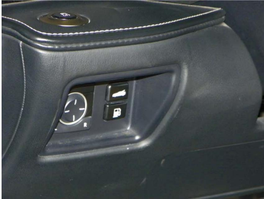
An override for this switch is provided in case this button does not function such as would be the case if the vehicle has a discharged battery. The override cable is located under a removable trim piece on the rear package tray.
