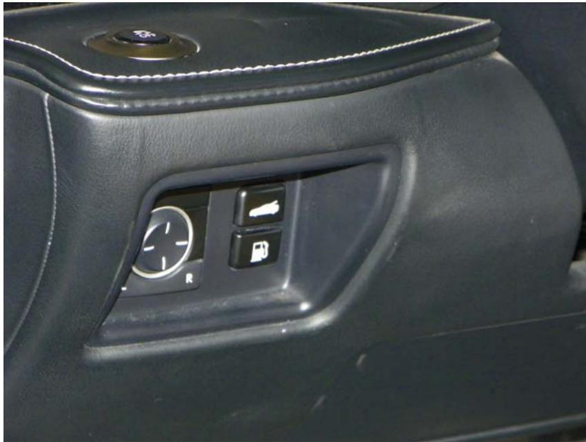
If the fuel filler door is inoperative due to a discharged battery or other trouble, there is an override in the cargo area on the left side behind the trim piece that covers the battery. Access to the cargo area can be obtained by depressing the cargo area release button above the fuel door release button on the dash. If the cargo area cover does not open when the button is depressed, refer to the override procedure listed on page 20.
