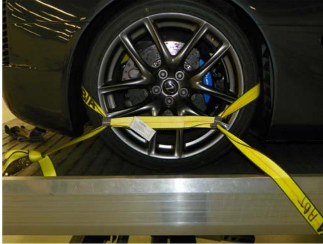
Clearance around the wheel is limited and careful routing of straps is needed to avoid contacting brake lines and wheel speed sensor wires, especially on the back side of the front wheels.
