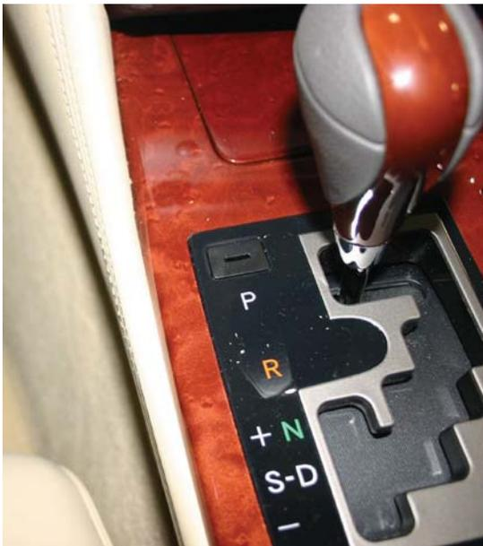
*(Figure 6 Shifter with access Plug in Place)*
