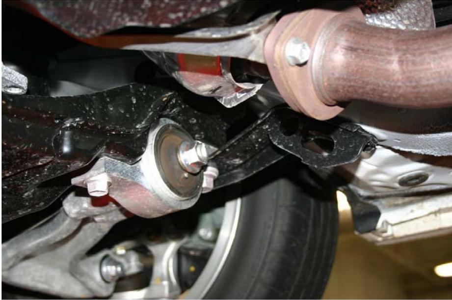
*Figure 3 (front tie down slot right side)*
