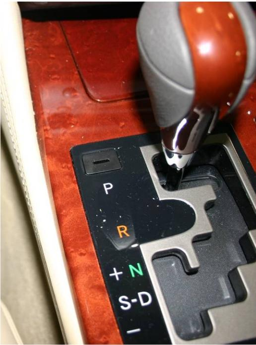
*(Figure 5 Shifter with access Plug in Place)*
