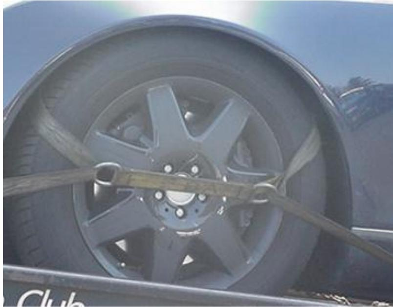
If nylon straps are not available, there are “T” hook slots in the unibody structure of the vehicle that can be used to secure it during transport. The tow truck operator must ensure that the ignition is not switched on at any time the vehicle is secured to the tow truck using the “T” hook slots as this may activate the adaptive suspension system on these vehicles.
