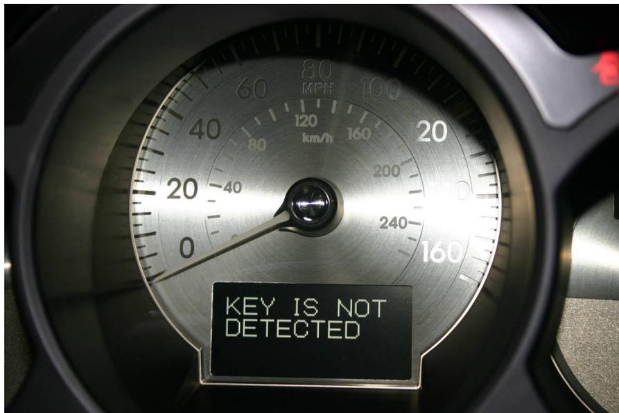
If this is occurring on a vehicle you encounter, ensure the vehicle is in “PARK”, hold the key fob against the chrome ring around the “ENGINE START STOP” button, depress the brake pedal then depress the “ENGINE START STOP” button to start the vehicle. If the vehicle starts, ensure the operator knows to hold the key fob against the chrome ring to start the vehicle and then direct the operator to take the vehicle to the closest Lexus dealer to have the problem repaired.
