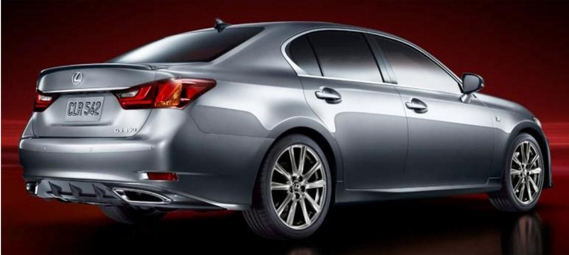
The 2013 Lexus GS Series vehicles have limited clearance on the front valance under the front bumper so it is recommended that a towing dolly should be installed under the trailing wheels when towing these vehicles with a wheel lift.
