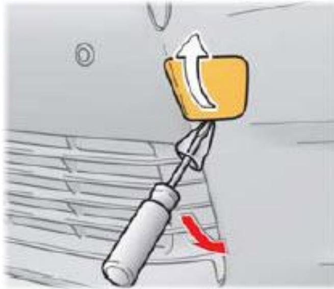
To install the eyelet correctly on this vehicle, start by carefully removing the eyelet receiver cap from the front bumper. If a sharp, metal object like a screwdriver is used as shown, use a cloth or piece of paper to protect the painted surfaces from scratches.
