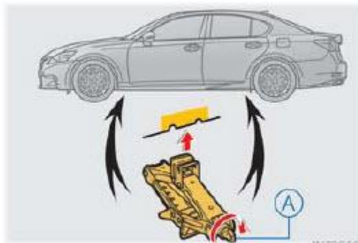
Place the jack in its proper location. Observe all standard jacking precautions and ensure that the vehicle is on firm, level ground. As the jack comes in contact with the vehicle body, ensure that it is contacting the correct location on the vehicle. Continue lifting to raise the vehicle high enough to change the tire.
