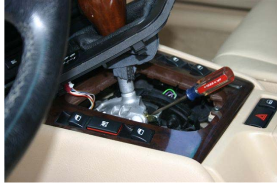
Use screwdriver type tool to lift interlock cam upward.
