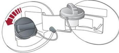
The fuel filler door can be opened when the vehicle is unlocked by pushing it in slightly. There is no emergency release for the filler door.
