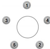
**Incrementally Torque Lug Nuts in the Pattern Shown Above to:
