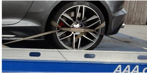
**Caution:** Do not over tighten the wheel straps or the vehicle may be damaged. Make sure no metal portions of the strap contact the wheel. Avoid scratching any surfaces with the wheel straps.
