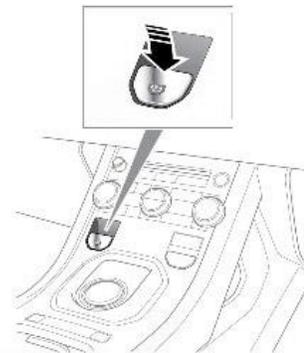
At this point, the vehicle should be in Nutral with the parking brake released, and can be loaded onto the car carrier.
