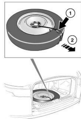
**Caution:** When removing the tire from the rear cargo area or trunk, prevent scratches or other damage by protecting the bumper and other painted surfaces with a fender cover.
