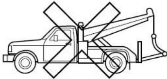
**Slingbelt towing is not an approved procedure. Vehicle damage may occur by this means.**
