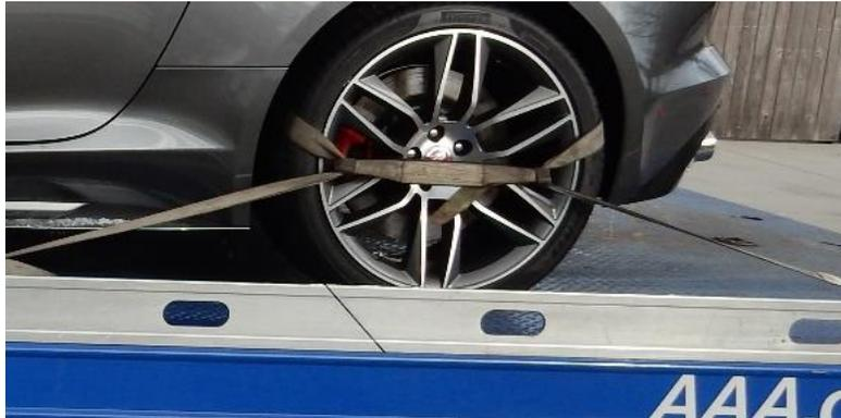
Only wheel straps should be used to secure the vehicle for transport. Damage may occur if wheel straps are not used. When the vehicle is in its loaded position on the flatbed with the bed still in the deployed position, secure the vehicle to prevent it from rolling by chocking the wheels and attaching one wheel strap to the wheel closest to you. Follow all normal loading procedures to tie down the rest of the vehicle and secure it for safe transport.
