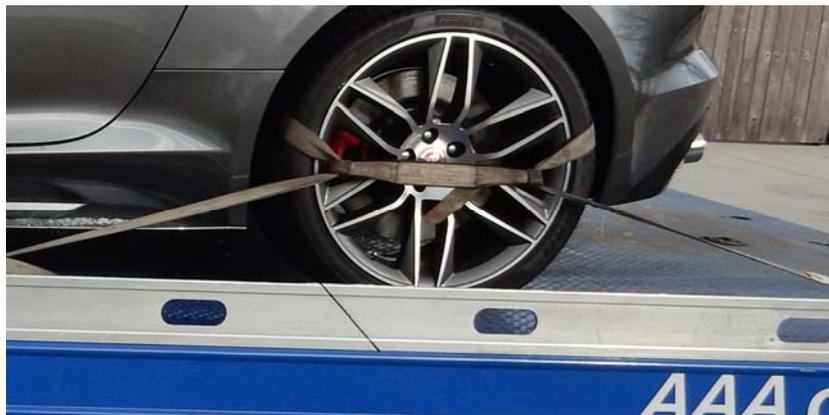
When the vehicle is in its loaded position on the flatbed with the bed still in the deployed position, secure the vehicle to prevent it from rolling by chocking the wheels and attaching one wheel strap to the wheel closest to you. Follow all normal loading procedures to tie down the rest of the vehicle and secure it for safe transport.
