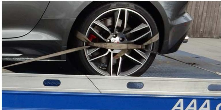
Only wheel straps should be used to secure the vehicle for transport. Damage may occur if wheel straps are not used.
