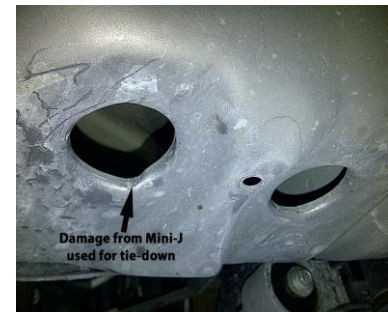
Outer hole damaged during tie down
