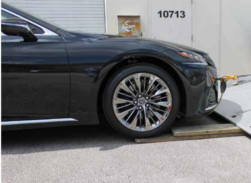
Utilize as much ramping as required to reduce the approach angle and retain adequate ground clearance at both the front and rear of the vehicle.
