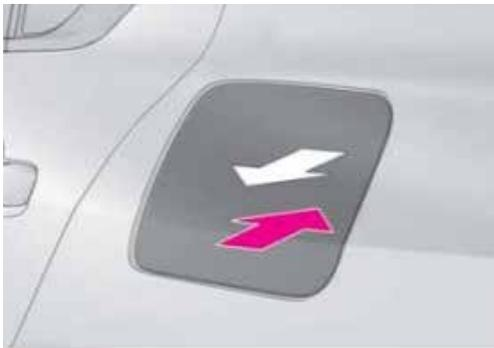
Take care not to damage the vehicle's finish during refueling. The fuel-filler door release is a push-lock design that requires the vehicle's doors to be unlocked for it to open. Press the rear edge of the fuel door about half way down to open the fuel filler door. After fueling and replacing the fuel cap, close the fuel door and press it again to lock the door closed.
