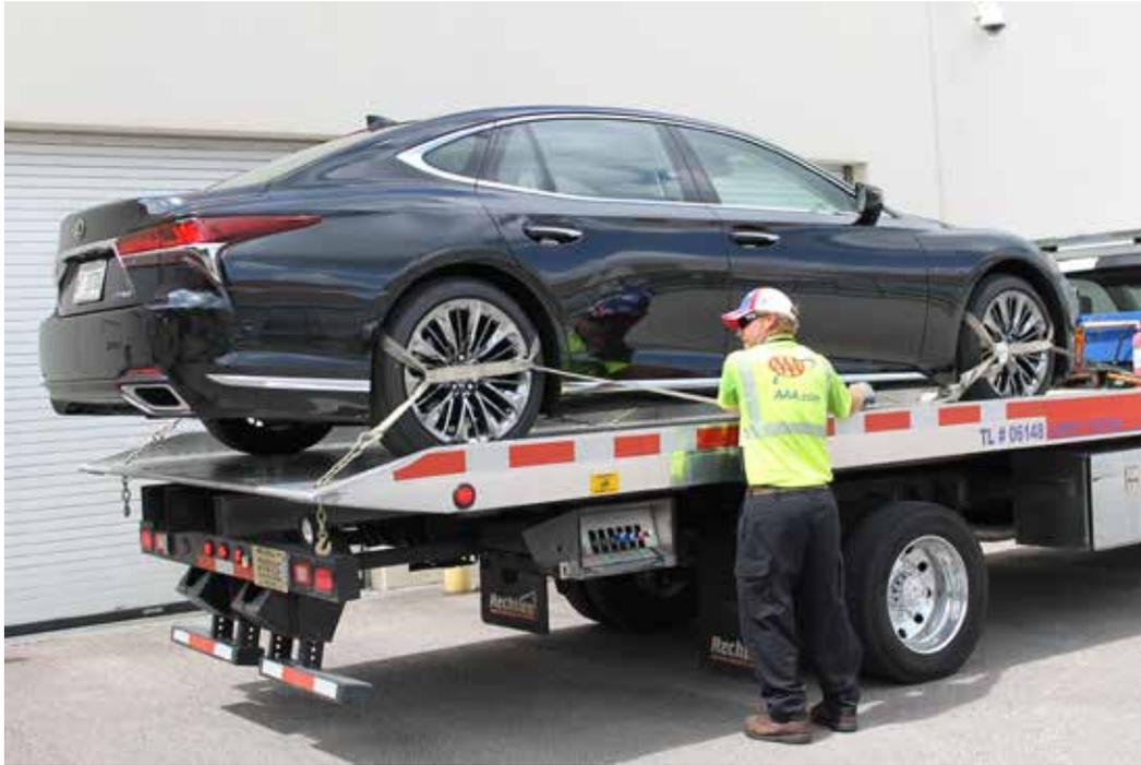
When the vehicle is in its loaded position on the car carrier with the bed still in the deployed position, secure the vehicle to prevent it from rolling by chocking the wheels and attaching one wheel strap to the wheel closest to you. Continue to secure the vehicle.
