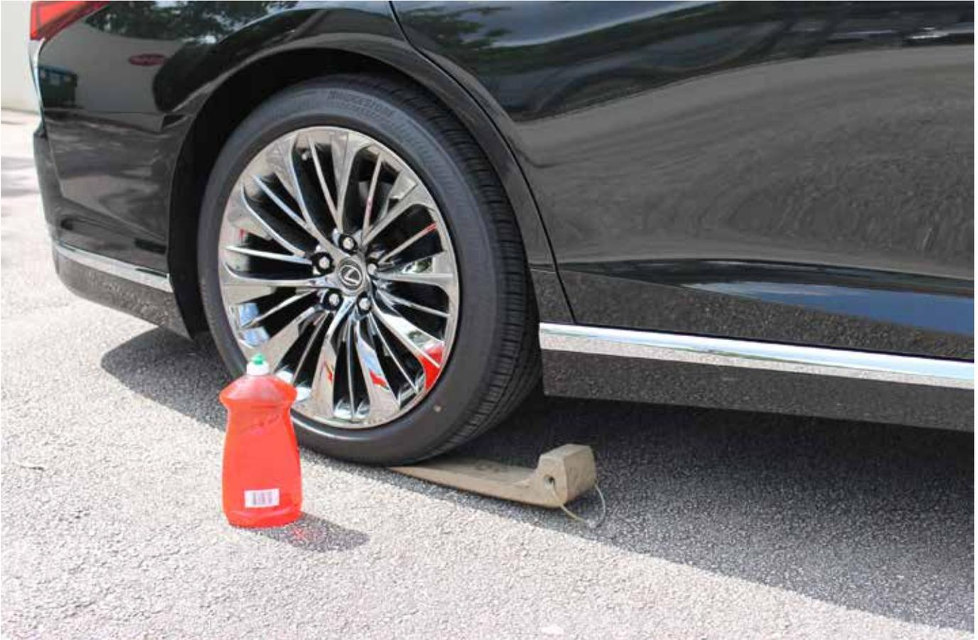
In the event Nutral cannot be selected or a failure with the parking brake mechanism causes the wheels not to roll, wheel dollies such as “GoJaks” or tire skates can be used on the non-rolling wheels to assist with loading the vehicle. Care must be taken when installing tire skates or GoJaks because of the limited clearance around the wheels and between the vehicle and the ground.
