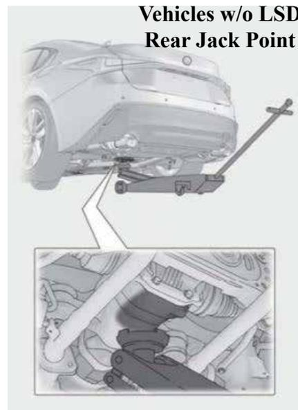
The jack needs to be of the low profile design in order to fit under the vehicle. Use of a rubber pad on the jack saddle is recommended to prevent damage at the contact point of the vehicle.
