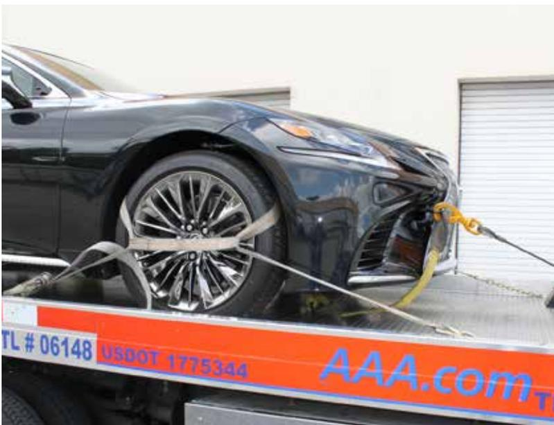
Clearance around the wheel is limited and careful routing of straps is needed to avoid contacting brake lines and wheel speed sensor wires, especially behind the front wheels. Careful routing of the straps is also important to avoid contact with the painted surfaces of the vehicle.
