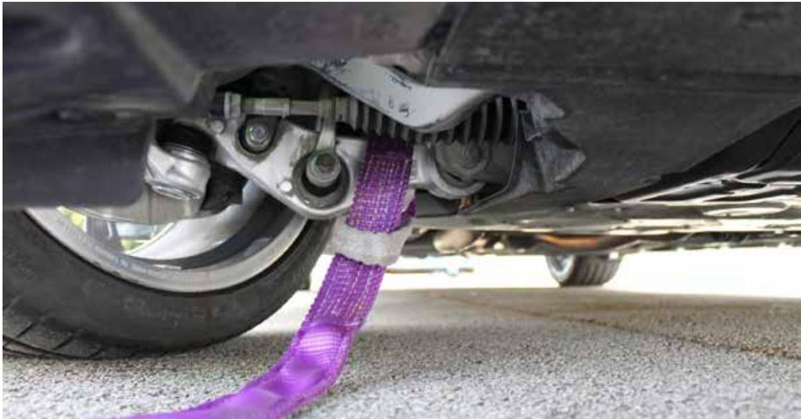
It is highly recommended to attach a secondary backup nylon strap to the vehicle. This is a precaution in the event the eyebolt attachment should fail. Using a short nylon strap, wrap the lower control arm and attach the other end to the winch line hook. This strap will remain slack and will only be utilized as a securing device if the eyebolt attachment fails.
